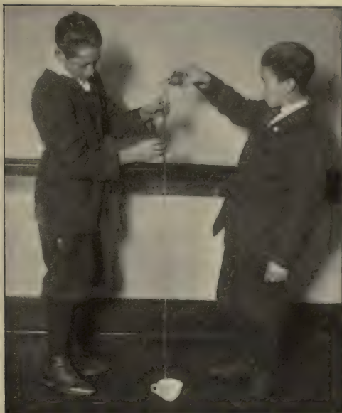
FIG. 152. Filling the barometer tube with mercury.
